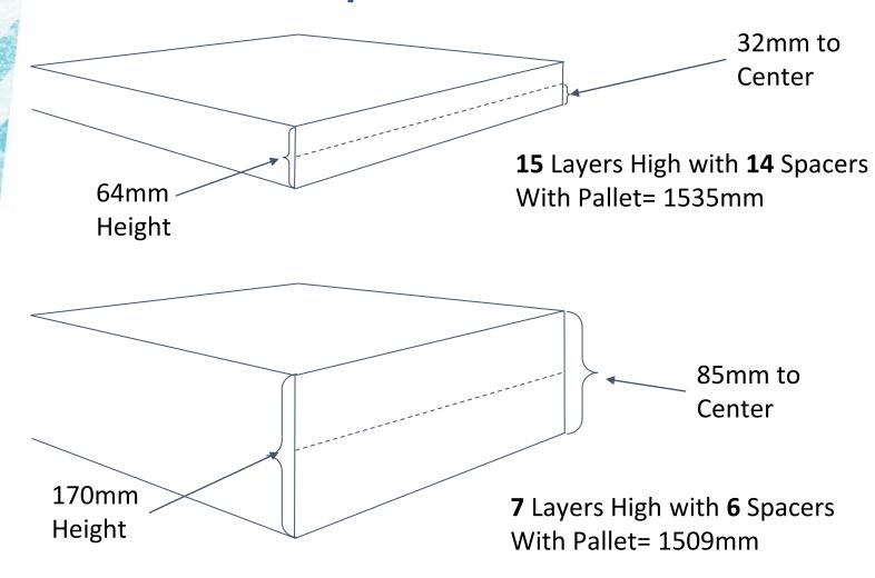
Taller Cases Reduce the Number of Layers, Which In Turn Reduces the Number Spacers Utilized. Therefore the Number of Air-Flow Paths are Reduced. Case Height Consideration #3 Combination of #1 and #2
