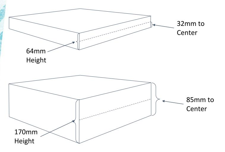
Taller Cases Drive Greater Distance to Center, Which Slows the Freezing at the Center of the Case.
