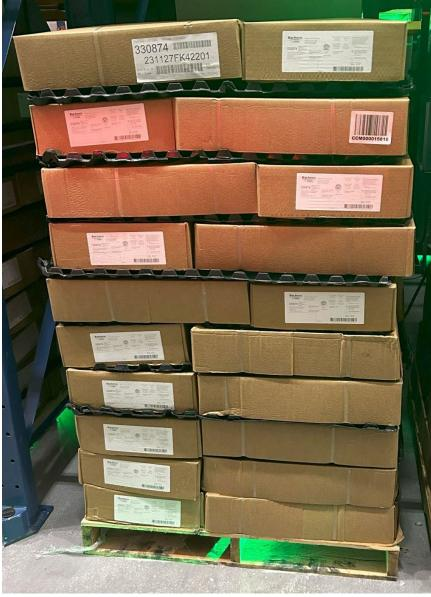
The top 4 layers have good air passages. As the weight increases with each layer, the spacers are crushed and no air is able to pass through the pallet. Spacers should be replaced every 3-4 years.
